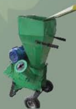
Agri Waste Chipper Machine Capacity = 300 kg per hour
